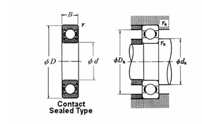
High quality Deep groove ball bearing with contact rubber seal on one side from the world leader NSK, the worlds largest ball bearing manufacturer offering unparalelled quality. The unique & patented NSK DDU rubber seal features market leading technology, keeping contaminants and moisture out of the bearing while retaining the high class lubricant inside
